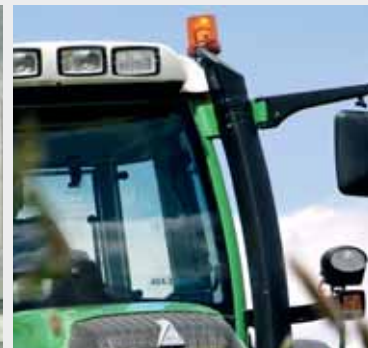
Additional Xenon work lights; rotating beacon
