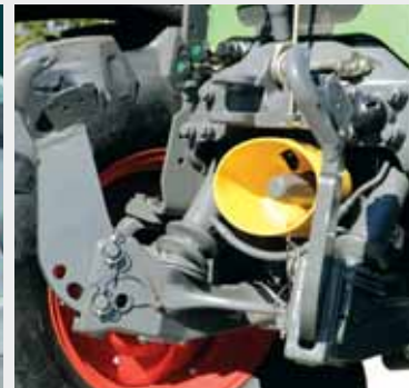
Integral front power lift and front PTO implements
