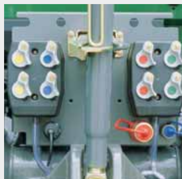
Double-sided connect-under-pressure couplings; external hydraulic connection (load sensing)
