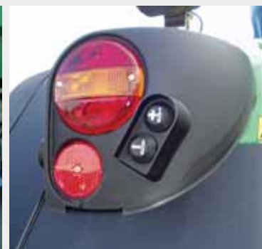
External control for hydraulic control unit at rear
